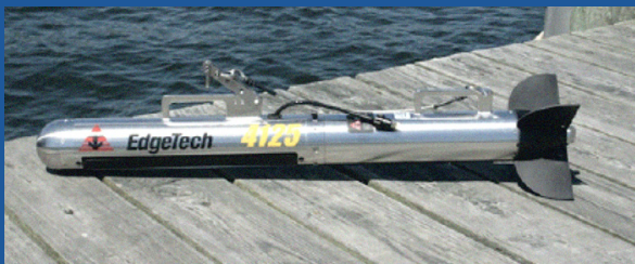
Side Scan Sonar (Foto: T&A Survey)
